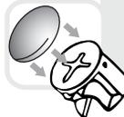
Al finalizar el ajuste de los conectores, proceda a poner las tapas adhesivas / When you finish the adjustment of the connectors, proceed to put the cover tapes
